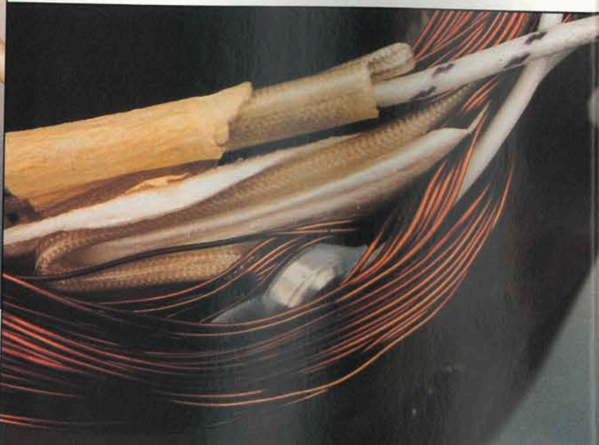
Figure 4, above and to the right, shows a thermal protector used in a single phase motor.
